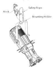
• Please use qualified safety-rope, which can hold at least 10 times the weight of the fixture. You must only use safety-ropes with quick links with screw cap. Pull the safety-rope through the hole on the bottom of the base and over the trussing system etc. Insert the end in the quick link and tighten the fixation screw. A safety rope which already hold the strain of a crash or which is defective must not be used again.
